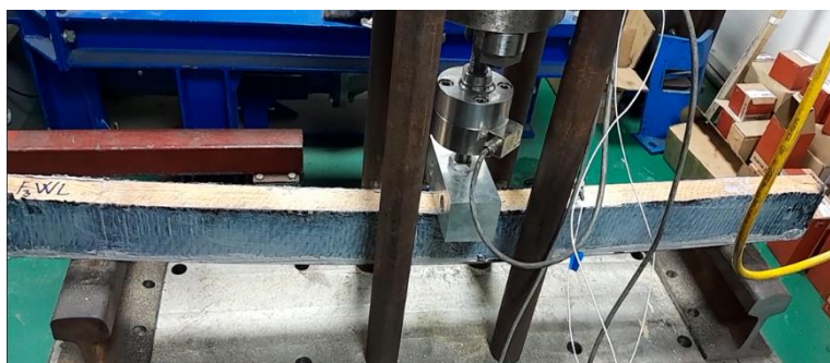
Figure 10. Bending test of the reinforced beach beam with carbon fiber fabric (in U-shaped) and one carbon fiber plate, F_3WL
