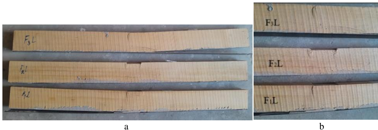
Figure 8. Reinforced beech beams with a carbon fiber plate F_1L , F_2L , F_3L after bending test (a), failure mode detail (b)
